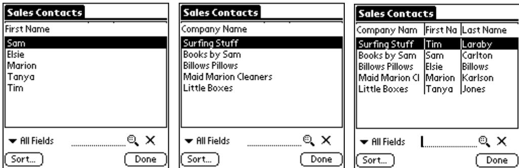
In the first picture above, the Display Key field is the first field on the form, which happens to be a customer's First Name. This field does not provide the user with much information, and so in the second picture, the Display Key field is changed to Company Name, a field which helps the user select which record he or she needs.
