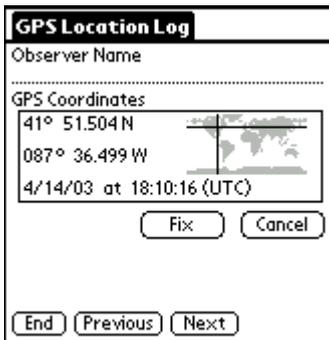
In order to use the GPS (Global Positioning System) Custom Control module, the handheld user will need an external GPS device that can attach to the handheld, or a Bluetooth-enabled GPS device or a handheld with a built-in GPS receiver.
