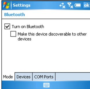
Step 1: On the Mode tab, make sure that Bluetooth is switched on.
