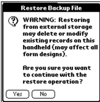
7. A Restore Backup File screen warns you that performing a restore may delete or modify existing records. This might occur if records were changed without being backed up, or if records were changed on the PC. This is why it is recommended to backup the Forms database on the PC before performing a restore.
